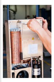
c. Check wiring and controller state
