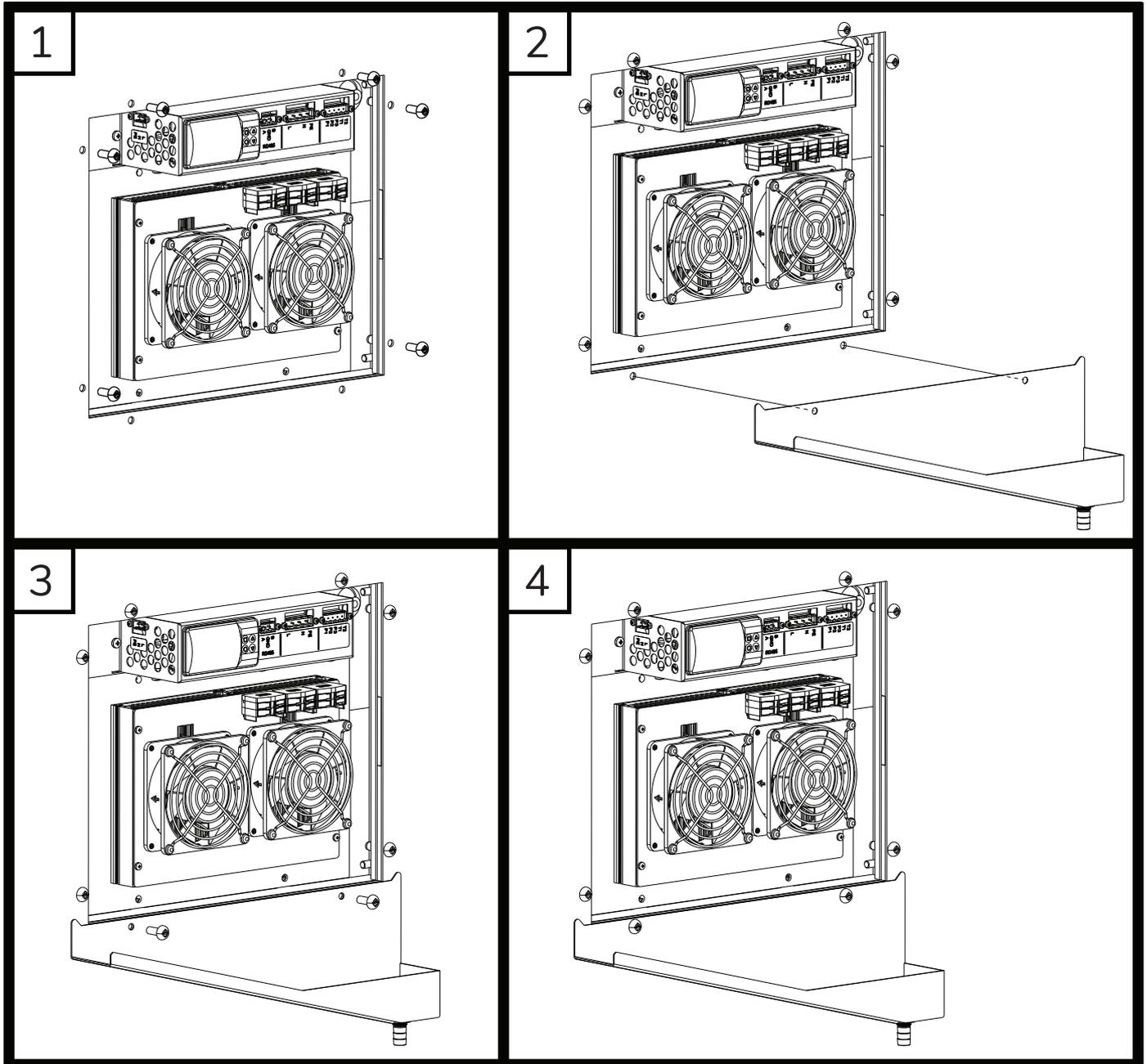
1. Mount Thermoelectric unit to the enclosure as instructed in the unit manual except for the bottom screws needed to fasten the condensate tray.
